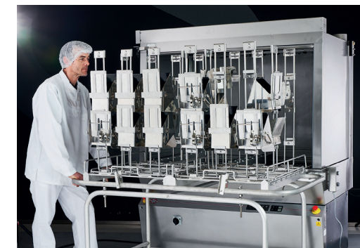
The trolley with the scales components safely fixed is rolled to the front of the JEROS ACE system.
