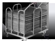
When the system stops, the tray wagon containing the clean trays is removed and an empty wagon can be put into place. The system is now able to continue cleaning more trays.
